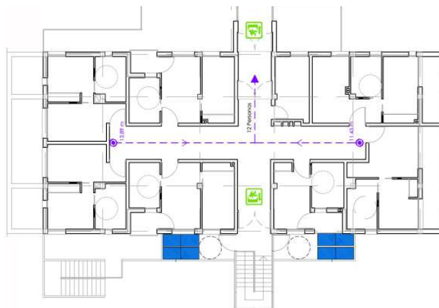
Evacuation refuge areas in the day centre at Tres Cantos, Madrid.
